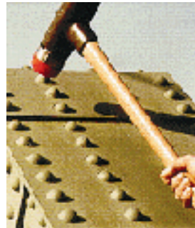
Instrumented sledge hammer used in modal testing of the stator.
